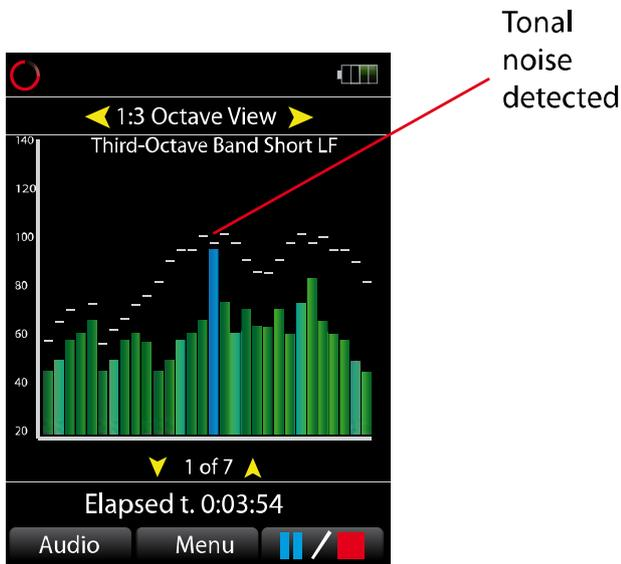
If the ISO method is used, the tonal noise detection will only be shown on the A-weighted screens (graphical and numeric). If the Cirrus improved method is used, the tonal noise detection is shown on both the Z and A weighted screens (graphical and numeric).
