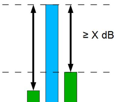
When a tone is detected using the ISO 1996-2:2007 Annex D method, it is highlighted in blue on the A weighted graphical screen and also the A weighted numeric screen.
