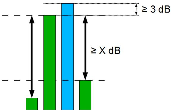
When a tone is detected using the Cirrus improved method, the appropriate band is highlighted on both the A and Z weighted screens.
