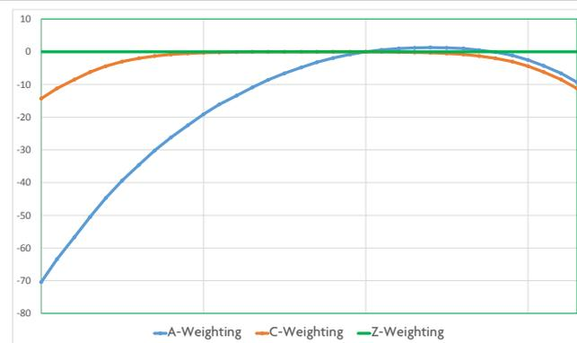
This graph provides a visual representation of the different frequency weightings. The x-axis represents the frequency; the y-axis represents the attenuation level in decibels. Attenuation, in acoustic terms, is a measure of the energy loss in sound propagation.
