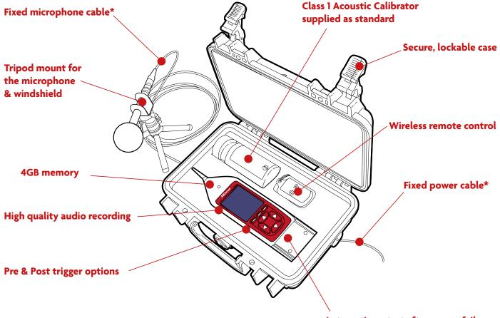
\*Cables can be replaced if they get damaged. The user cannot remove the power or microphone cable.
