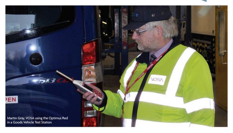
The Optimus Red boasts a high resolution colour **OLED** which simplifies the use of the instrument and makes viewing the noise results a lot easier.
