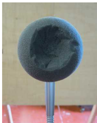
Figure 9: windshield 'B' with cutout
