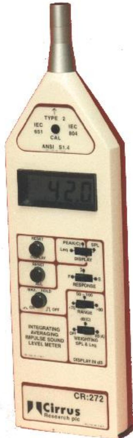
In the right position, marked >80 the instrument measures levels in the range 80 to 140dB.
