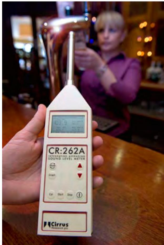
logging or storage of measurements in the instrument. Downloading measurements to a software program allows measurements to be stored for later reference, to be used in risk assessment reports or for more detailed analysis and noise exposure calculations.
